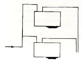
Cooling water drains must be separate.
